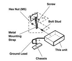
Reinforce the head unit with the metal mounting strap (not supplied). Secure the ground lead of the unit to a clean metal spot using a screw (\*) already attached to the vehicle's chassis.
