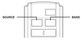
2 Press the BAND button on the CDA-9827/CDA-9825 or the RUE-4187 to activate the CD Changer Selection mode. 3 The CD Changer Selection mode remains active for 8 seconds after step 2 is performed. Press the BAND/ TEL. button until the desired CD Changer indicator appears on the display.
