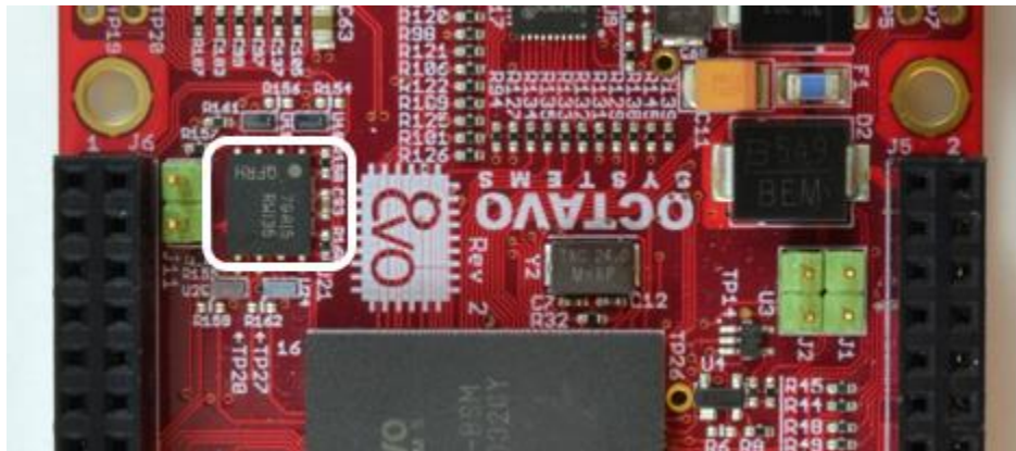
Figure 36: NOR flash on board
