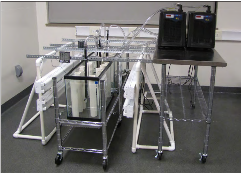
Figure 2.8 Aquaria setup with lighting, chilling, and aeration system in place
