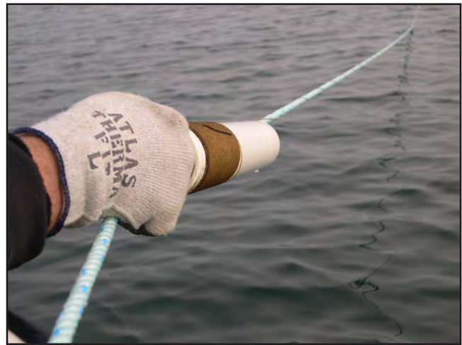
Figure 5.5 Long line threaded through spool; crew tensioning long line
