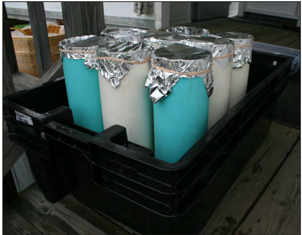
Figure 5.3 Settling tubes and spools packed for transport before ice is added around tubes
