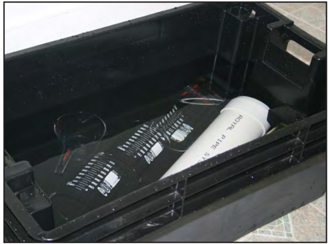
Figure 4.20 Equipment soaking overnight in bleach and deionized water solution
