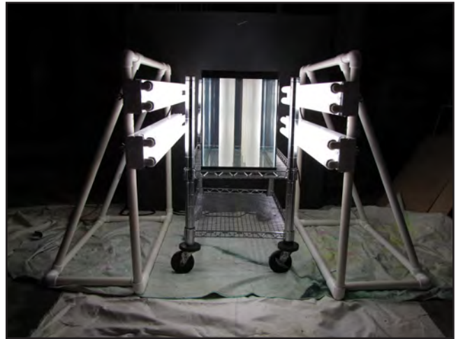
Figure 2.3 The light bank setup fabricated by OA to administer light to the growing spools
