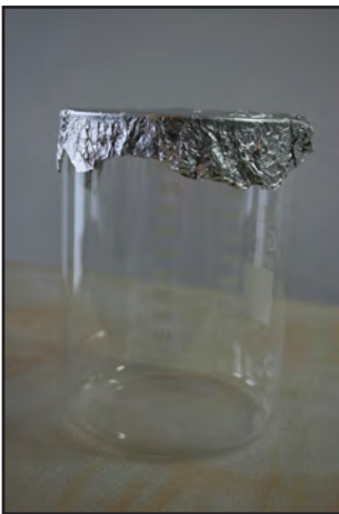
Figure 4.21 Glassware with an aluminum foil cover to prevent contamination
