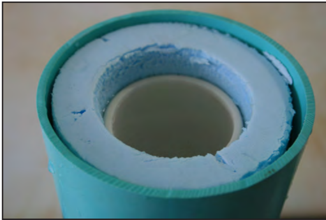
Figure 5.2 Styrofoam ring keeps spool from moving inside settling tube during transport.
