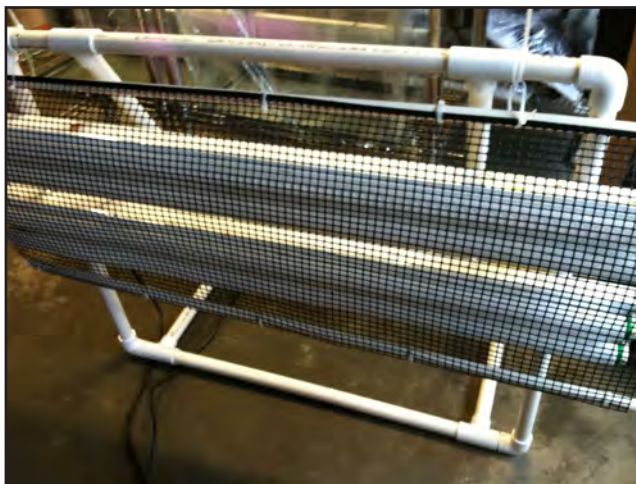
Figure 2.5 Wide mesh screen used to create light levels of 55 \mu\text{mol m}^{-2} \text{s}^{-1}
