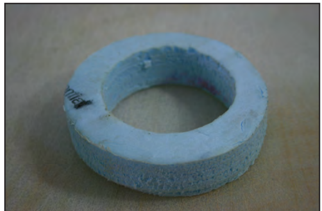
Figure 5.1 Styrofoam ring cut to fit around spools inside of settling tubes for transport to farm site
