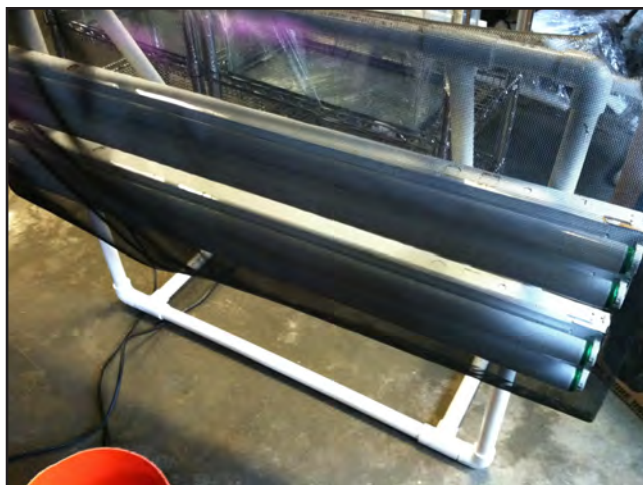
Figure 2.4 Fine mesh screen used to create light levels of 20 \mu\text{mol m}^{-2} \text{s}^{-1}
