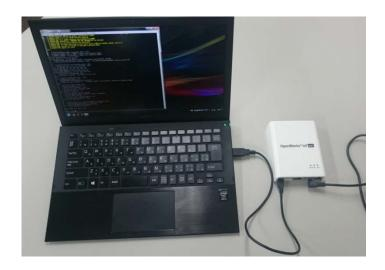
In the case of a Windows PC, connection to a USB port will automatically install a USB serial driver (if Windows PC is connected to an Internet environment).
