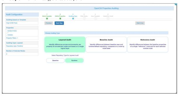
In the above example, we want to perform a so-called "layered audit", which means that we want to compare property values across multiple installations and report differences where one or multiple values are different. E.g. if an Integration Server Core fix level is "3.2" in DEV, but "3.1" in TEST and PROD, then we will see that in the result.
