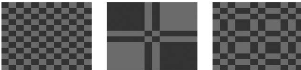
Figure 9-5 GL_REPEAT , GL_CLAMP_TO_EDGE , and GL_MIRRORED_REPEAT Modes
