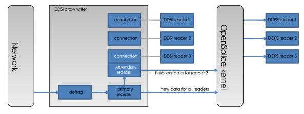
Fragmented data first enters the defragmentation stage, which is per proxy writer. The number of samples that can be defragmented simultaneously is limited, for reliable data to Internal/DefragReliableMaxSamples and for unreliable data to Internal/DefragUnreliableMaxSamples.
