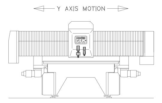
The y axis is the movement of the carriage, carrying the ultrasonic knife cutting head and inkjet printhead or labeler units, across the length of the crossbeam.
