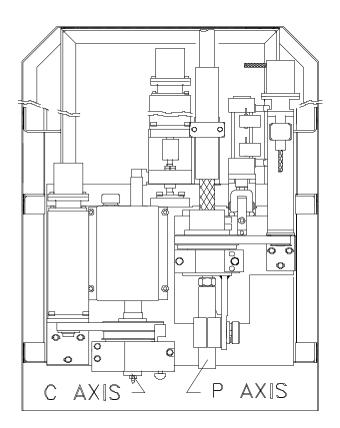
The c axis is the rotational movement of the cutting blade.
