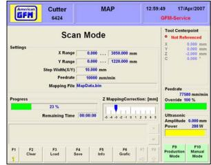
mapping sensor in the Z direction. When the scanning cycle is complete, choose F4 Save to save the mapping data to the mapping file. Lastly, choose F3 Load to load the mapping file to the CNC. The View Mapping utility is also available by choosing F6 Graphic.
