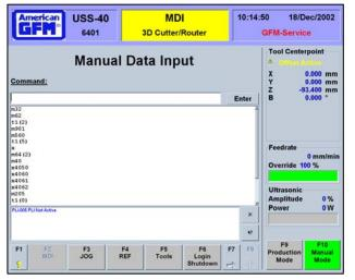
The History button will open a drop-down menu showing the most recently entered commands in the command line. Clicking on a command in the history menu will enter the command into the Command: window. Pressing enter will send the command to the CNC.
