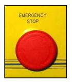
Several E-stop pushbuttons are located around the machine and on the AGFM CNC 6000 operator control console. Pressing any of these emergency stops will cause the machine movement to cease, and the machine will remain inactive until the emergency has been cleared. Note, however, that power is not removed from the CNC when an E-stop button has been depressed. All power will be removed from axis servo drive systems and pneumatic solenoids with any emergency stop condition.
