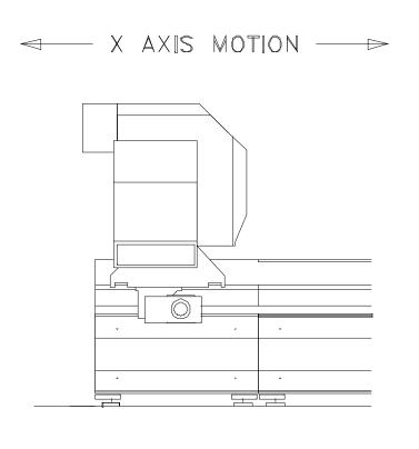
The x axis is the movement of the crossbeam along the length of the machine.
