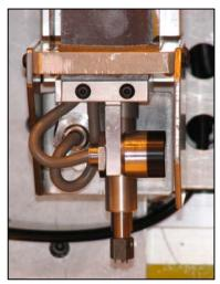
Material), the CNC reads the sensors again and stores the values as the "Ending Value". The CNC then calculates how much deviation occurred during the M36 pull-out and automatically makes a correction to XY axis compensate for the belt deviation. This correction occurs after every M36 so that every window is accurately cut. This system is accurate to within +/- 0.20mm.
