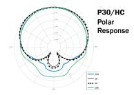
sponse results in less phase problems on the sides of the microphone and there are fewer phase cancellations when using multiple mics placed close together. This new microphone technology also provides more rejection of unwanted sounds from the rear of the microphone and more gain before feedback in live sound applications.
