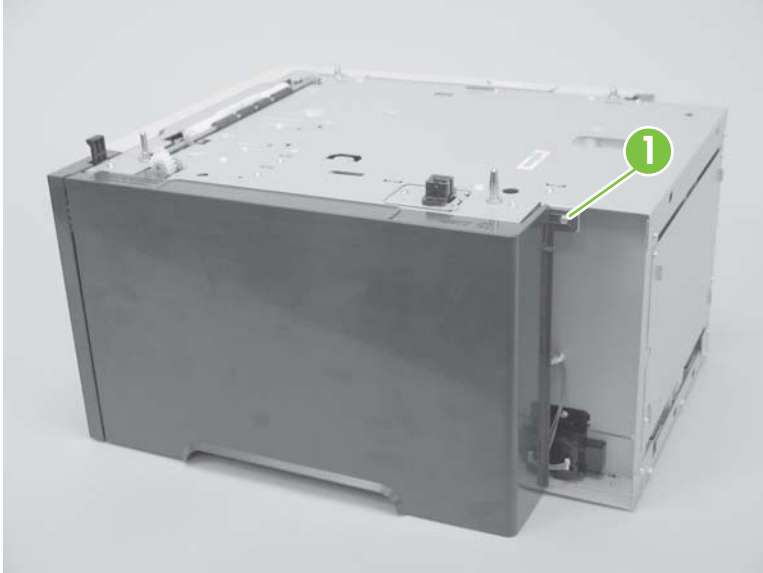
Figure 6-132 Remove the 1,500-sheet feeder right-side cover (1 of 2)
