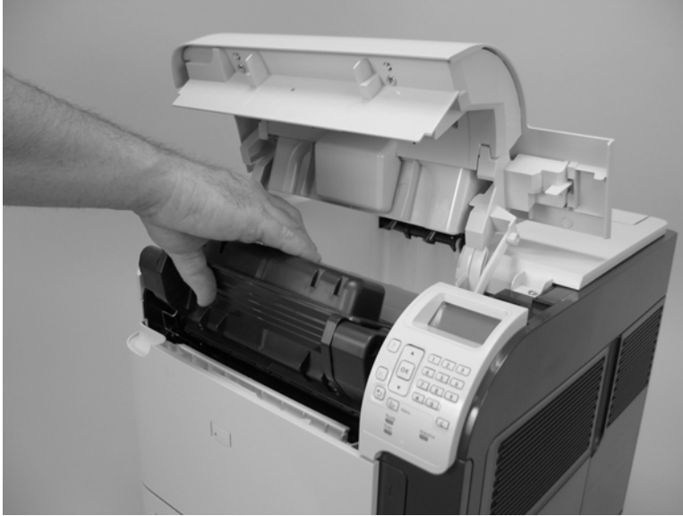
Figure 6-6 Remove the print cartridge (2 of 2)
