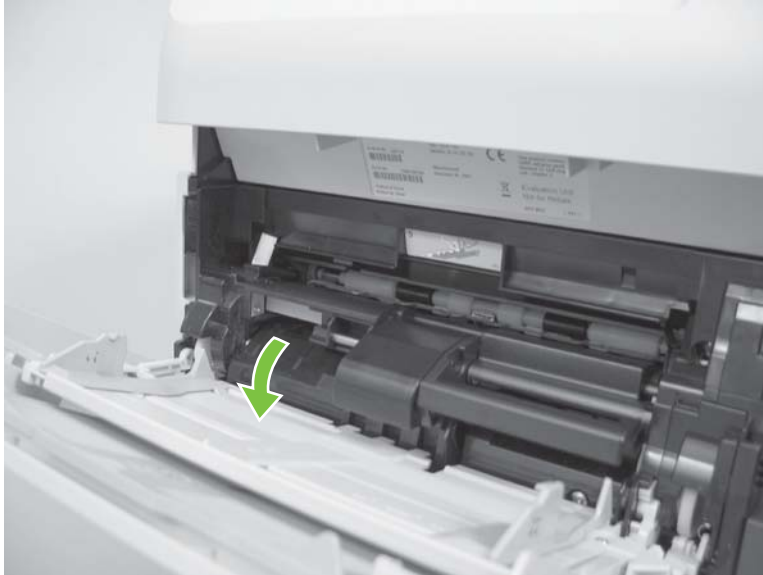
Figure 6-31 Remove the Tray 1 separation roller (1 of 3)
