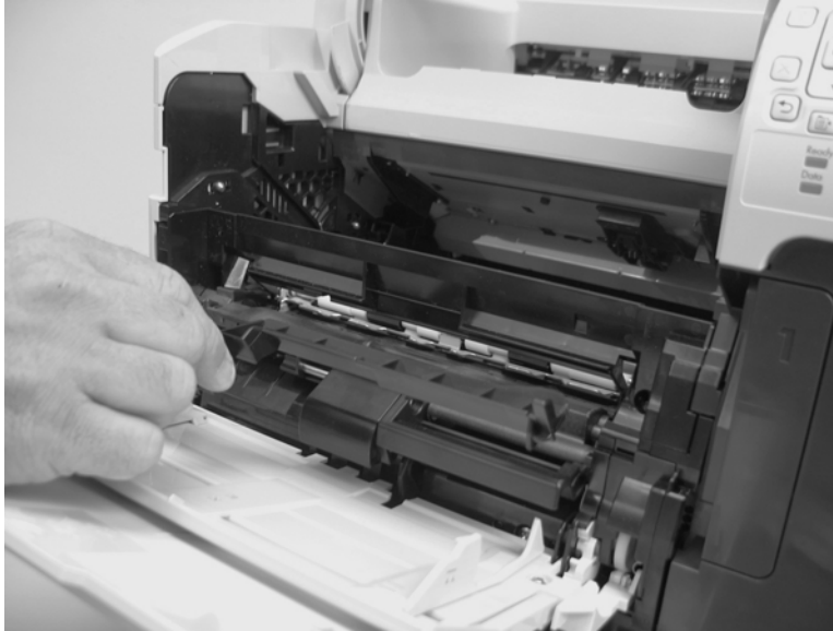
Figure 6-15 Remove the front accessory covers (1 of 2)
