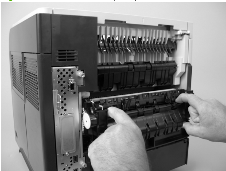
Figure 6-24 Remove the fuser (2 of 2)
