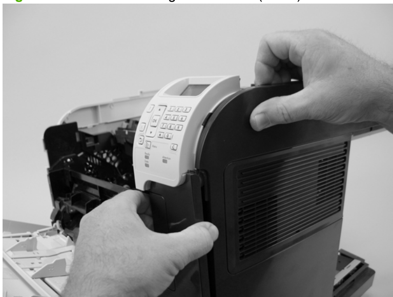
Figure 6-43 Remove the right-side cover (2 of 3)
