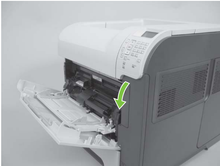
Figure 6-16 Remove the front accessory covers (2 of 2)
