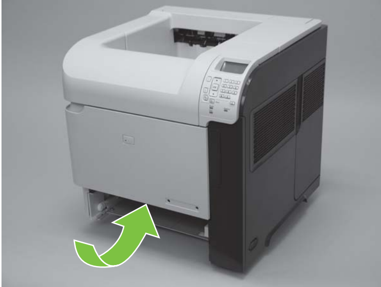
Figure 6-11 Remove the Tray 2 separation, pickup, and feed rollers (3 of 4)
