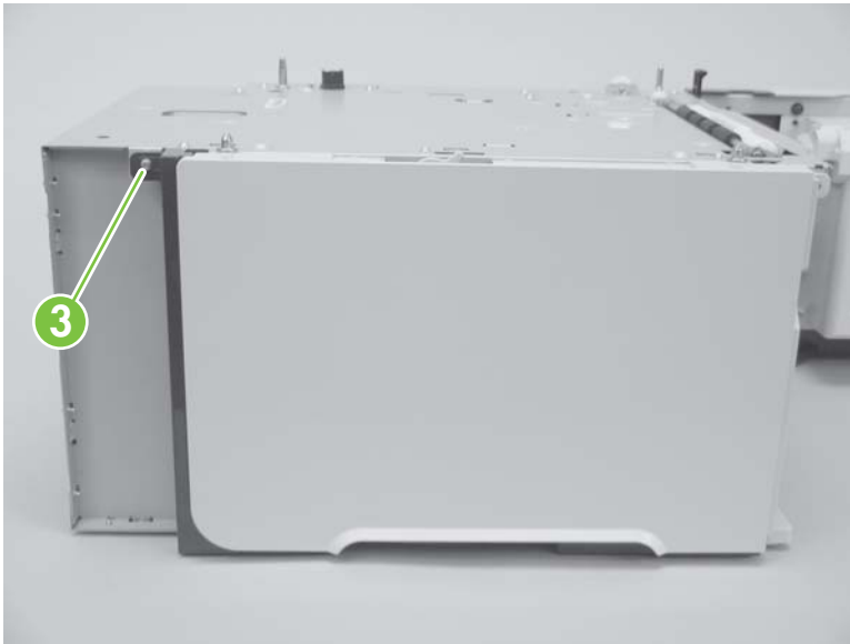
Figure 6-137 Remove the 1,500-sheet feeder left-side cover (4 of 5)
