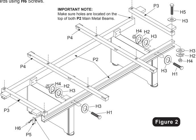
**Note: P5** Main Beam End Boards must be flush or slightly lower than top of **P3** End Slats.
