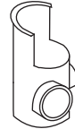
Left Corner Pocket NOTE: Attach this pocket on same end as P14 Apron with Ball Return Opening 1 Pc
