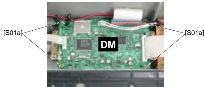
[S01]: Bind Head Tapping Screw-B 3.0x8 MFZN2W3 (WE774300) Bタイト + BIND (Photo 3)
