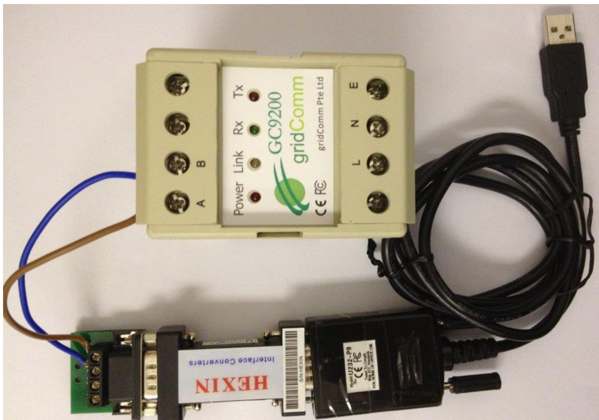
Figure 2 – GC9200 Connection with a RS485-RS232-USB Cable
