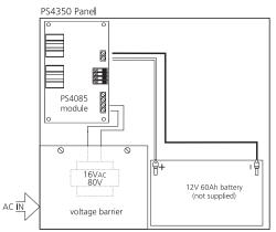
INSTALL BATTERY AND AC WIRING AS SHOWN ABOVE IMPORTANT: A minimum of  $1/4^{**}$  (7mm) separation must be maintained at all points between battery/primary AC wiring and all other wiring and connections.
