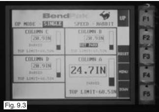
NOTE: When the PCL-18 is not loaded with a vehicle the Speed should be set to Rabbit mode or a fault condition may be detected. See page 29 for Troubleshooting and Faults.
