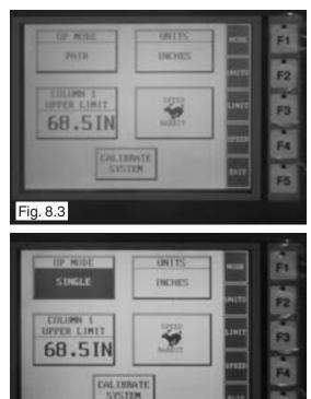
7. Pressing **UNITS** or F2 (Column A Control Panel only) allows the operator to set the unit of measurement to either Inches (See Fig 8.5) or Millimeters. (See Fig 8.6)
