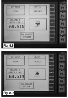
10. Pressing **CALIBRATE SYSTEM** (Column A Control Panel only) will set the current height of the lift carriages as the 0 point or ground level. (See Fig 8.10 and 8.11)
