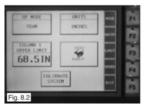
6. Pressing **OP MODE** or F1 allows the operator to control he movement of the entire system in Team mode (See Fig 8.2), Columns A and B in Pair mode (See Fig 8.3) or Column A by itself in Single Mode (See Fig 8.4)
