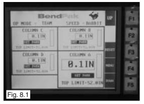
If any of the Column heights are any value over than 0.1 IN or 0.2 IN press the "**DOWN**" or F5 button. If the heights still do not read correctly see Maintenance section for calibration instructions.
