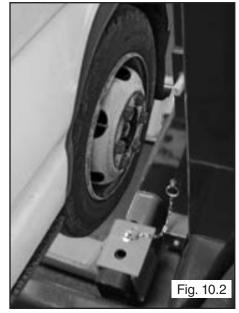
6. Lower the Column and adjust the fork arms by pushing the arms until they touch or are as close to the tire as possible. The lift should be parallel to the vehicle body without touching the body or other components of the vehicle. (See Fig 10.3)
