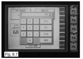
9. Pressing **SPEED** or F4 allows the operator to change the speed at which the lift will lower when the DOWN button is pressed. Rabbit mode (See Fig 8.8) allows for a quicker descent while Turtle mode (See Fig 8.9) allows for a slower, more precise descent.
