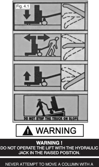
NEVER ATTEMPT TO MOVE A COLUMN WITH A VEHICLE LOADED ON THE ARM FORKS.
