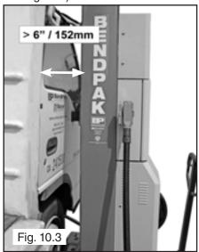
7. When all the Columns are properly positioned and the clearances around and above the vehicle are confirmed clear of obstructions, the Columns can be connected.
