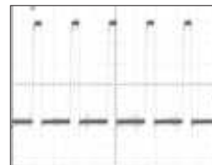
⑧ SC9002 17-pin (FORMAT MTRISCLK) H : 2 \mu sec/div V : 1.44V/div
