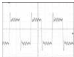
⑨ SC9002 25-pin (FORMAT MTRCLK) H : 40m sec/div V : 1.44V/div
