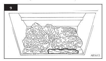
7.7 Place log E across from the rear of log A to log C on the right hand side. Again, there are cut-outs for location. The front of the log should sit on the front ash panels and should fit tight to log C. See diagram 10.
