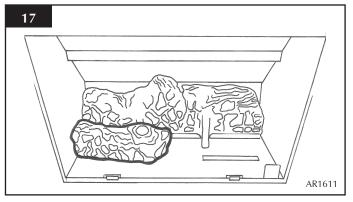
5.1 Place log C on the right hand side of the burner with the location bar on the underside of the log fully located in the long slot in the burner. Make sure the log is as far right as possible. See diagram 18.
