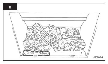
7.6 Place the second ash panel to the right of the first, with the pointed end of the panel fitting into the V shape. This panel should locate on the screw holes of the burner skin. Ensure that both logs are horizontal to the burner ports.
