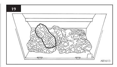
5.3 There are two ash panels which lay across the front of the burner skin. Place the panel with the flat edge facing the left side of the firebox. There are location holes on this log which fit over the screw holes of the burner skin.
