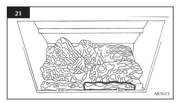
5.5 Place log E across from the rear of log A to log C on the right hand side. Again, there are cut-outs for location. The front of the log should sit on the front ash panels and should fit tight to log C. See diagram 22.
