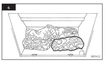
7.4 Place log D across from the rear log A to log B on the left-hand side. There are cut-outs in both logs for location. See diagram 7.
