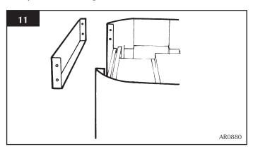
3.3.4 Locate the lower panels onto the lugs as shown. See Diagram 12.
