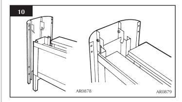
3.3.3 Secure the upper front panel using the 4 nuts and bolts provided. See Diagram 11.
