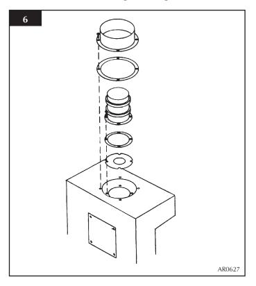
3.2.3 If the horizontal terminal is used assemble the required amount of vertical flue including the 90° elbow onto the stove. Drill through the fixing hole in the spigot using a 3.5mm drill and secure with the screw provided. Do not
