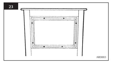
5.7 Offer the steel door fascia to the opening, inserting the two tags on the bottom of the frame behind the bottom panel. Swing the top of the frame up and hook the lugs on the back of the frame, over the top of the glass frame. See Diagram 23.
