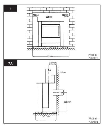
The above dimensions provide adequate clearance at the side and rear of the fire so that the controls can be reached.
