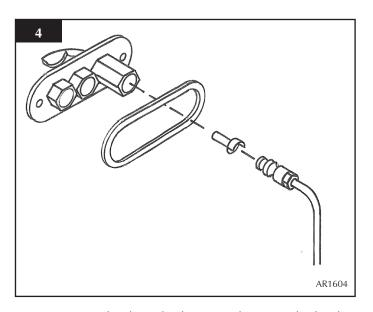
3.5 To remove the electrode, disconnect the ignition lead and undo the retaining nut. The electrode can now be removed, note the orientation of the electrode terminal when reassembling. See diagram 5.
