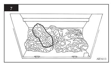
7.5 There are two ash panels which lay across the front of the burner skin. Place the panel with the flat edge facing the left side of the firebox. There are location holes on this log which fit over the screw holes of the burner skin.
