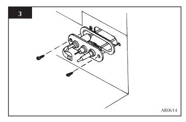
3.4 To remove the pilot injector, undo the compression nut on the pilot feed pipe and withdraw the injector which will be hooked onto the olive. When replacing an injector always make sure it is hooked onto the olive before inserting it into the pilot burner. See diagram 4.
