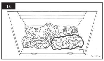
5.2 Place log D across from the rear log A to log B on the lefthand side. There are cut-outs in both logs for location. See diagram 19.
