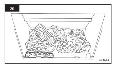
5.4 Place the second ash panel to the right of the first, with the pointed end of the panel fitting into the V shape. This panel should locate on the screw holes of the burner skin. Ensure that both logs are horizontal to the burner ports.
