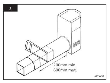
3.1.6 From outside, locate the flue assembly into the hole until the terminal is flat against the wall. Ensure the terminal is vertical. NOTE THE ORIENTATION OF THE TERMINAL. See diagram 3. Mark the four fixing holes, remove the terminal and drill the holes, inserting the rawplugs supplied.
