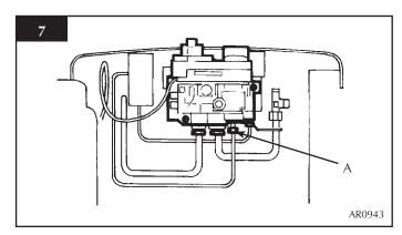
3.7 To remove the gasket, disconnect all the above components and withdraw the gasket. If it is damaged, replace with a new item. Always replace the gasket first when reassembling the pilot components.
