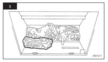
7.3 Place log C on the right hand side of the burner with the location bar on the underside of the log fully located in the long slot in the burner. Make sure the log is as far right as possible. See diagram 6.
