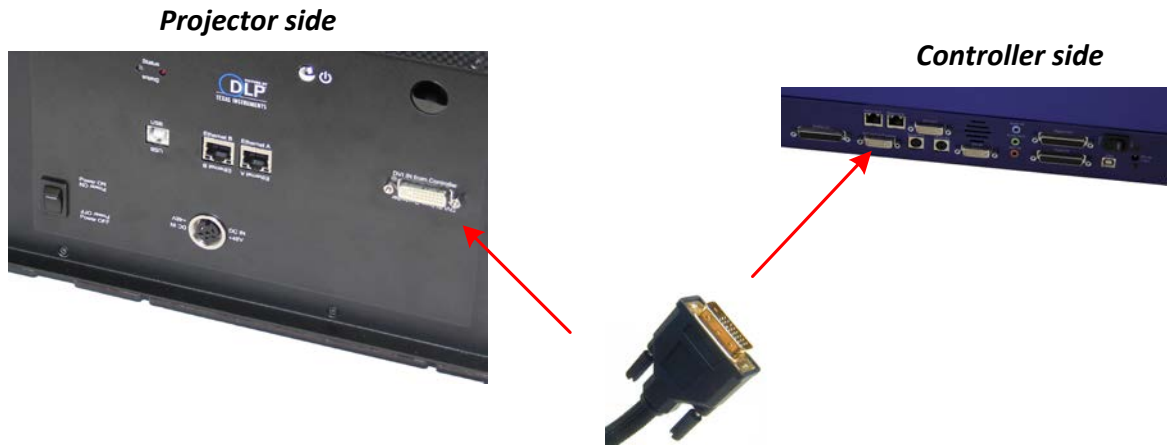
Figure 12 DVI cable between projector and controller
