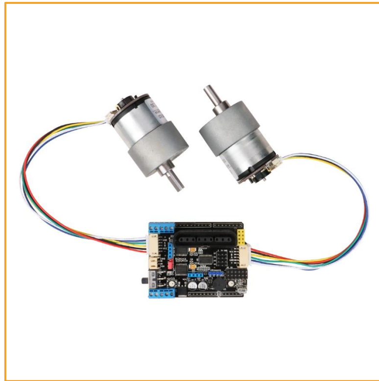
Figure 8-3 Coded motor connection diagram
