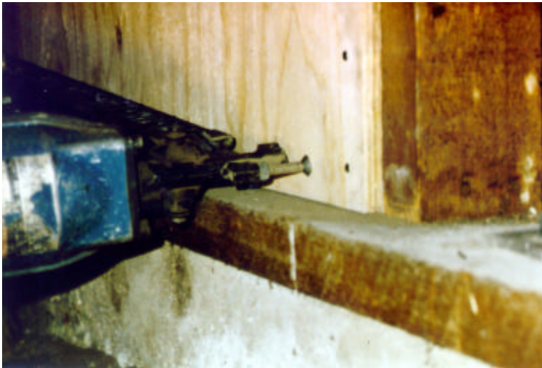
Fig. 3.43 Sample Nail Gun with Flush Attachment
