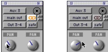
Linked (left) and unlinked (right) Output windows
