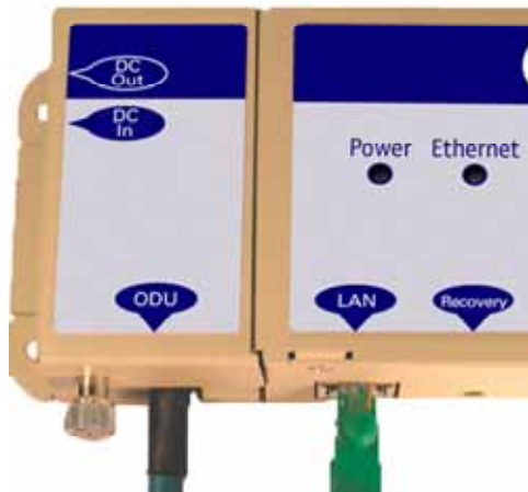
Figure 22 - Making the Network Connection at the PTP 400 Series Bridge PIDU Plus
