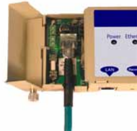
Step 2: Plug in the ODU to PIDU Plus Cable ensuring that it snaps home
