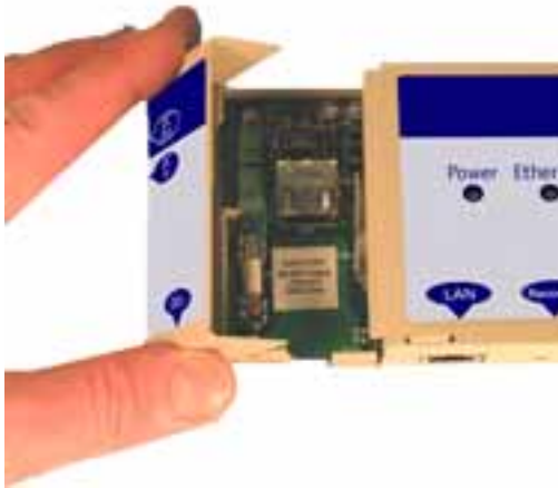
Step 1: Undo the retaining screw and hinge back the cover.
