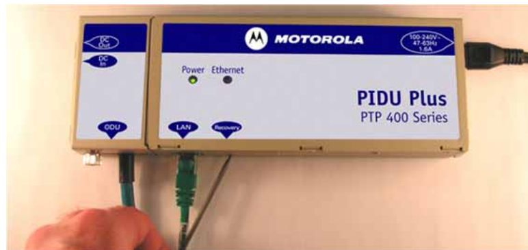
Figure 4 - PTP 400 Series Bridge Recovery Switch Location
