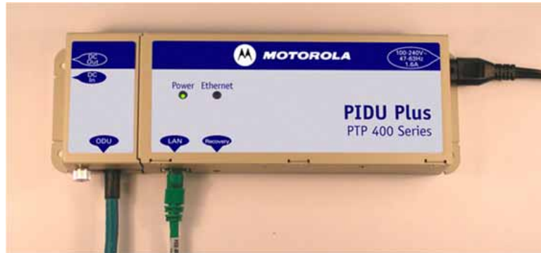
Figure 3 - Power Indoor Unit (PIDU Plus) – PTP 400 Series
