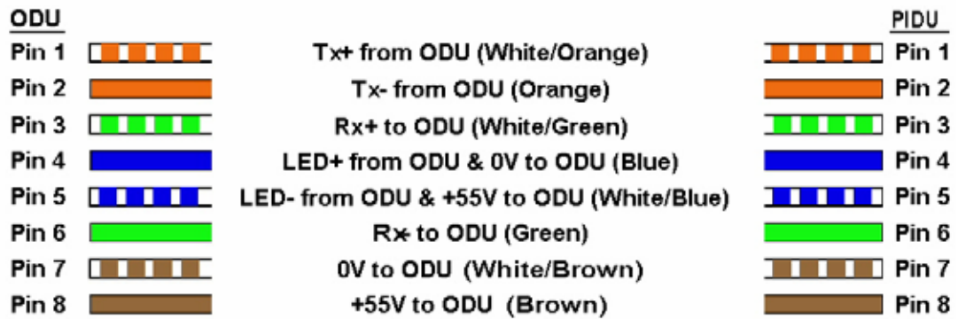
Figure 75 - ODU to PIDU Plus Connection Diagram
