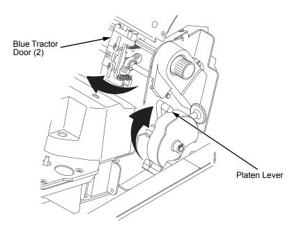
Figure 21. Preparing to Load the Ribbon
