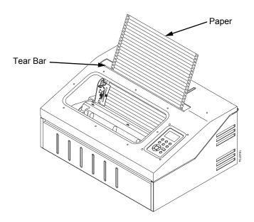
Figure 58. Paper Exiting the Top of the Printer
