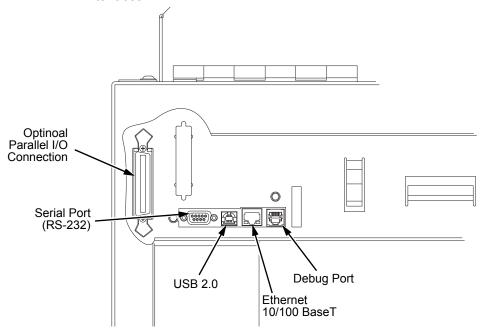
**Figure 25. Cabinet Model Interface Connectors**
