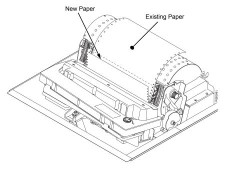
Figure 10. Loading New Paper into the Printer
