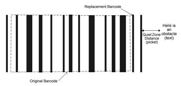
Center (factory default). The first attempted position of the center bar of the replacement barcode will be the same position as the center bar of the original barcode.
