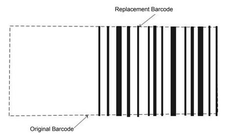
If the replacement barcode is larger than the original barcode, the replacement barcode will end at the right edge of the original barcode and extend past the left edge. Any form elements (text, graphics, or dots) immediately to the left of the original barcode, however, can force this first attempted placement to be modified. The replacement barcode will shift right to avoid obstacles on the left provided that there are also no obstacles on the right.
