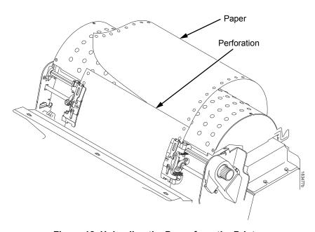
Figure 18. Unloading the Paper from the Printer
