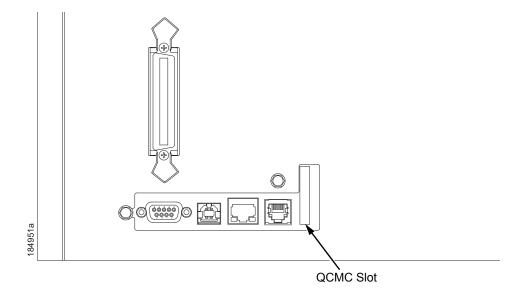
Figure 63. QCMC Slot on Back of Pedestal
