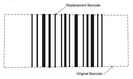
If the replacement barcode is longer than the original barcode, it will still be centered, but it will extend beyond the end of the original barcode on both the left and the right.
