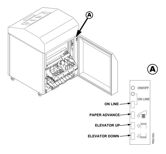
Figure 50. The Rear Control Panel
