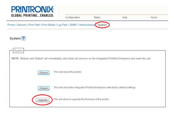
Figure 28. System Configuration Upgrade
