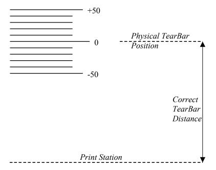
Figure 60. Correct Tear Bar Distance
