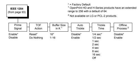
The IEEE 1284 interface is faster and more versatile than Centronics and supports bidirectional communication. Configuration of this interface is controlled from the host. Refer to "IEEE 1284 Parallel Interface" on page 255 for more details about the available modes (Compatibility, Nibble, and Byte).
