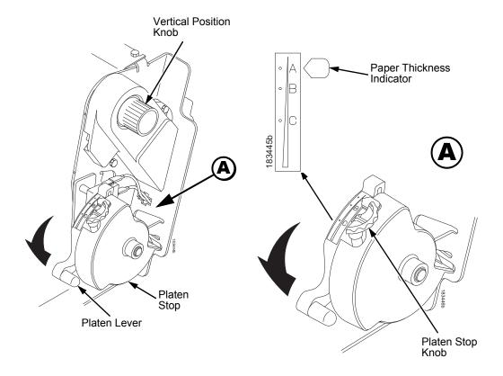
Figure 17. Adjusting the Platen Lever
