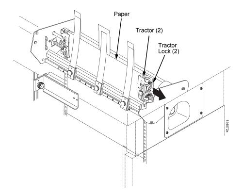
Figure 57. Adjusting the Horizontal Paper Tension
