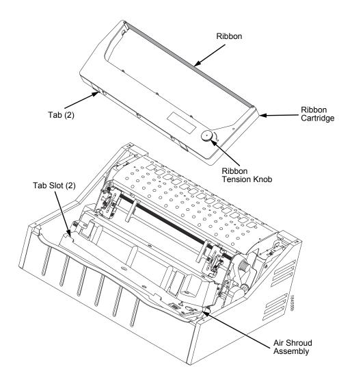
Figure 22. Installing the Ribbon Cartridge
