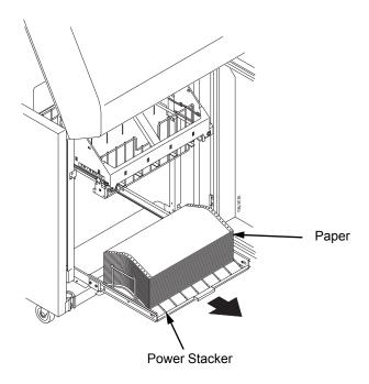
Figure 19. Removing Stacked Paper from the Printer
