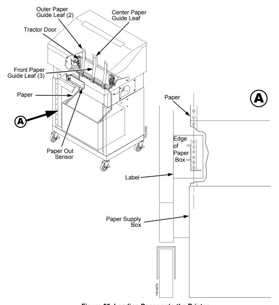
Figure 56. Loading Paper onto the Printer
