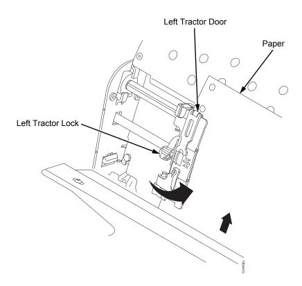
Figure 12. Loading Paper on the Left Tractor
