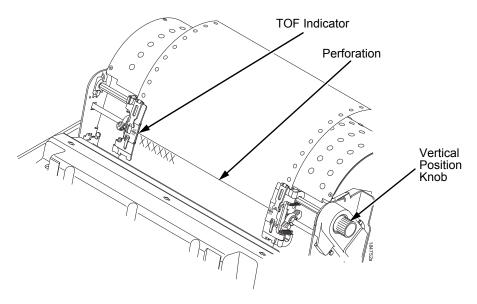
Figure 16. Aligning the Perforation with the TOF Indicator
