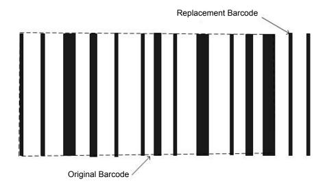
Any form elements (text, graphics, or dots) immediately to the right of the original barcode can force this first attempted placement to be modified. The replacement barcode will shift left to avoid obstacles on the right provided that there are also no obstacles on the left.
