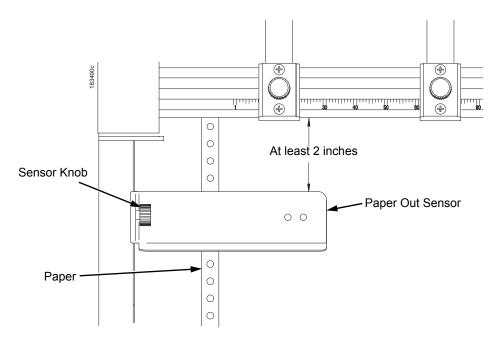
Figure 59. The Paper Out Sensor
