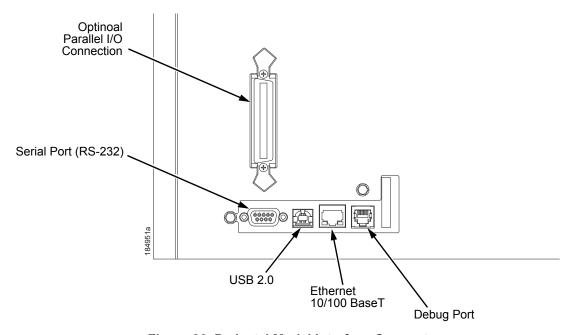
Figure 26. Pedestal Model Interface Connectors
