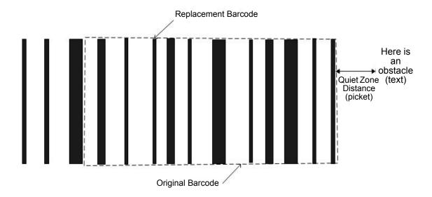
Right. The first attempted position of the rightmost bar of the replacement barcode will be the same position as the rightmost bar of the original barcode.
