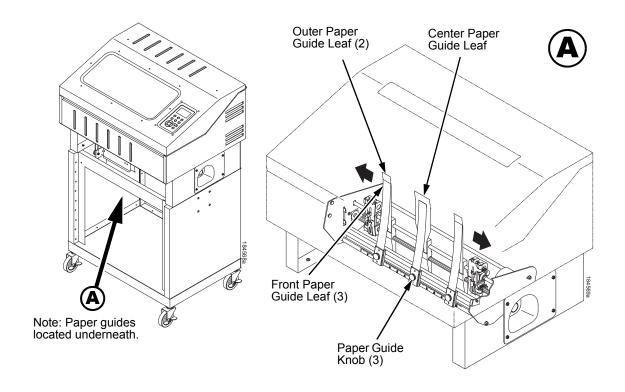
Figure 54. Adjusting the Paper Guides
