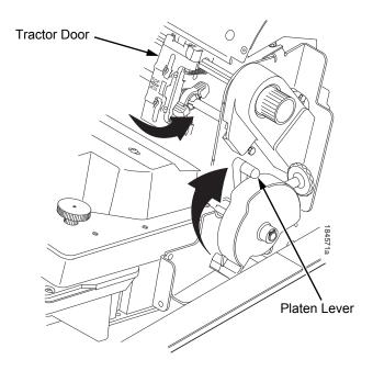
Figure 20. Completely Removing the Paper
