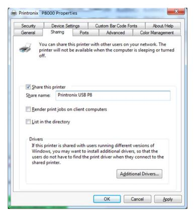
Figure 34. Setting Printer Properties Sharing Options
