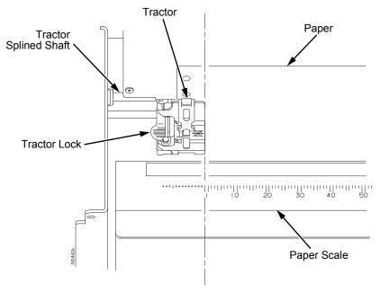
Figure 13. Positioning the Left Tractor to Avoid Damage
