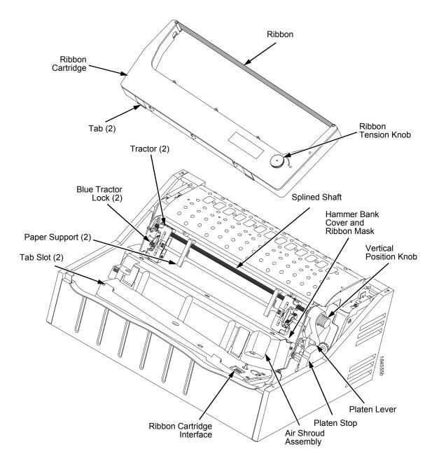
**Figure 47. Interior Printer Components**
