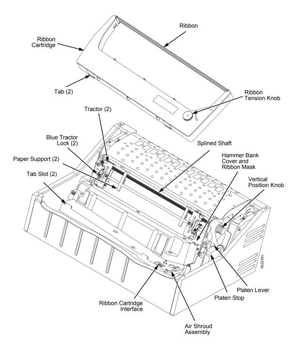
**Figure 7. Printer Component Locations**
