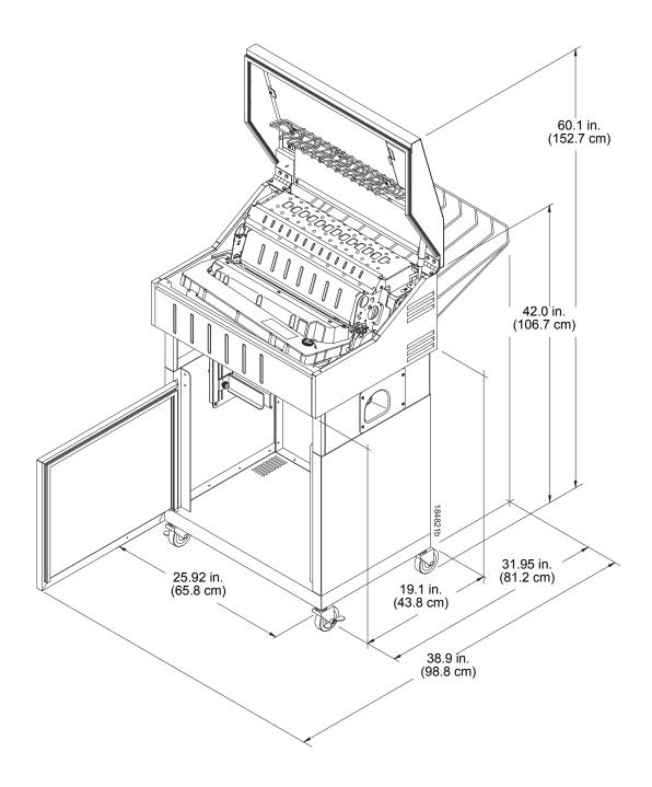
Figure 6. Zero Tear Pedestal Model
