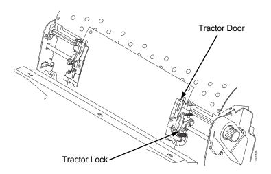
Figure 14. Loading Paper onto the Sprockets
