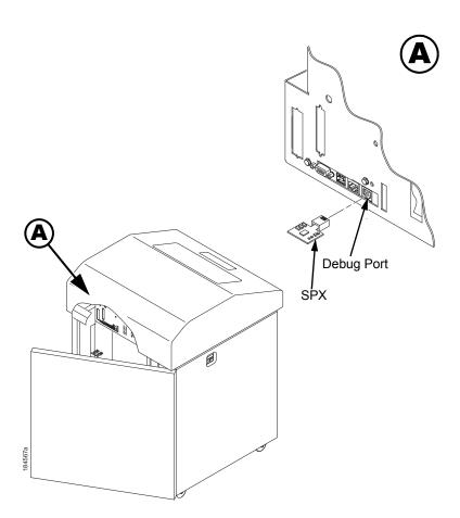
Figure 27. Inserting The SPX into the Debug Port
