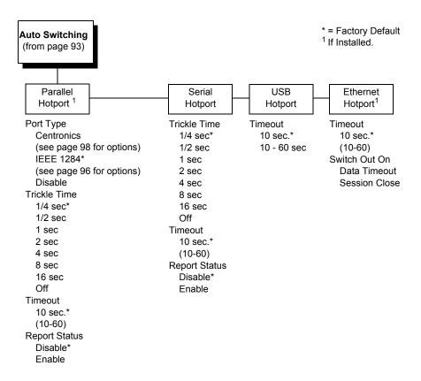
Auto Switching gives the printer the ability to handle multiple data streams sequentially. With Auto Switching, the printer can service hosts attached to the serial, parallel, USB, and Ethernet ports as if they were the only interface connected.
