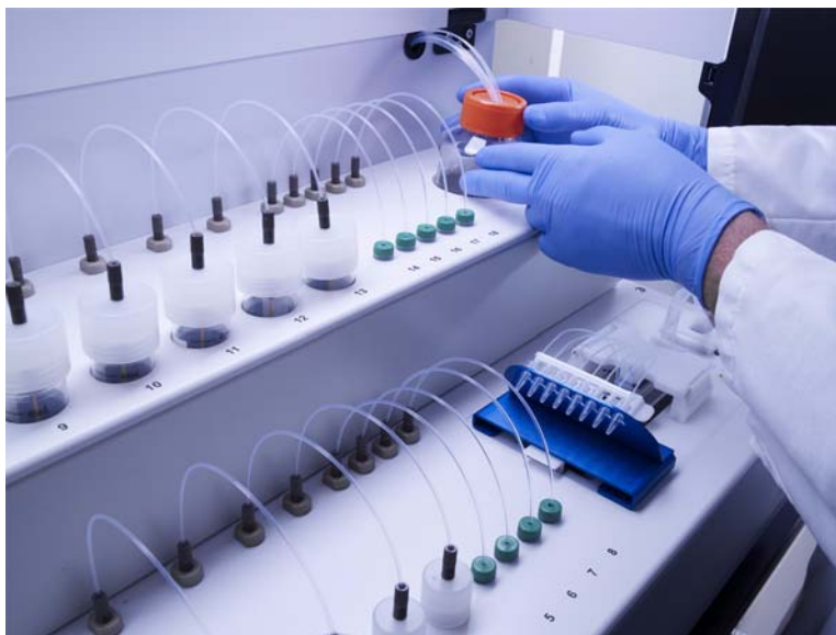
Figure 18 Liquid Waste Container on the Cluster Station
