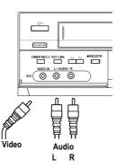
Connect your external source (for example: Video Camcorder) to the front input. To select A3 press **JINPUT SELECT AVJ** repeatedly. The sound will be recorded on
