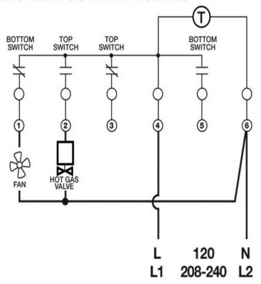
Hot gas defrosting with fan delay.
