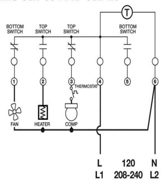
Electric heat defrosting with fan delay.
