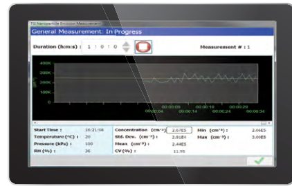
General Purpose Test Mode Display Output: Live strip chart of total solid particle number concentration with 1 Hz frequency and cumulative statistics.
