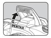
Switch between Auto discharge mode and Manual discharge mode (Flash ON) by pressing the **4UP** button while the built-in flash is popped up. If Auto discharge is set, **GUID** appears on the LCD panel.
