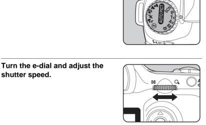
The shutter speed and aperture value are displayed in the viewfinder and on the LCD panel.
