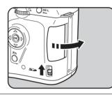
**2** Insert the card all the way with the SD Memory Card label toward the LCD monitor.
