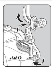
**2** Pass the other end of the strap through the other strap lug on the camera, then secure on the inside of the clasp.
