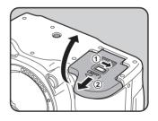
Insert the batteries according to the +/- indicators in the battery chamber.
