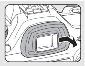
clearly even if you set the diopter adjustment lever, use the diopter correction lens adapter M. However, the eyecup must be removed to use this adapter. (p.188) Memo
