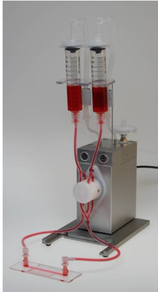
Figure 9: Correctly mounted Perfusion Set
