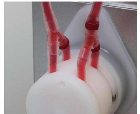
Figure 13: Correct order of Perfusion Set tubing
