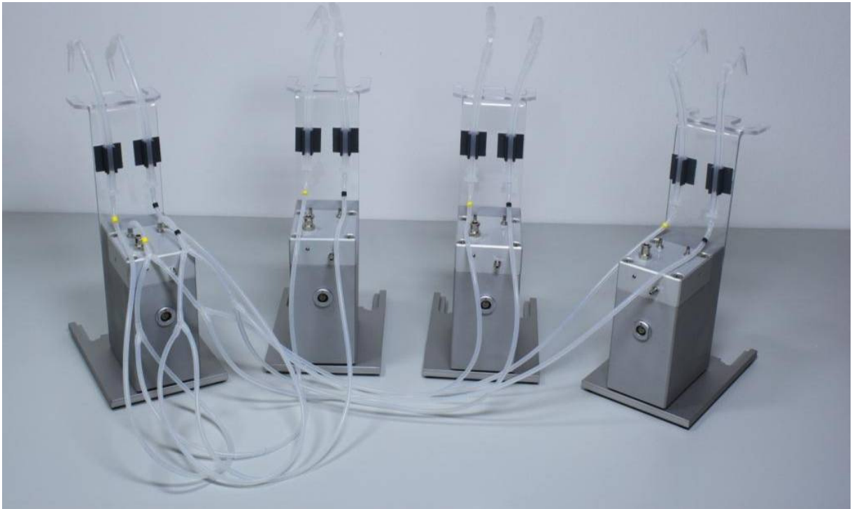
Figure 33: Air pressure connection with a setup using 4 Fluidic Units
