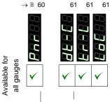
The name of the parameter is displayed as long as the key is pressed or at least for 1.5 s.
