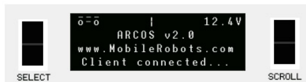
Figure 17. In normal mode, the LCD accessory displays operating status and client generated messages.
