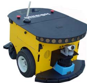
Figure 7. PowerBot™ carries over 100 kg of payload.
