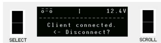
Figure 18. In interactive mode, the LCD lets you modify some operating features of the microcontroller.
