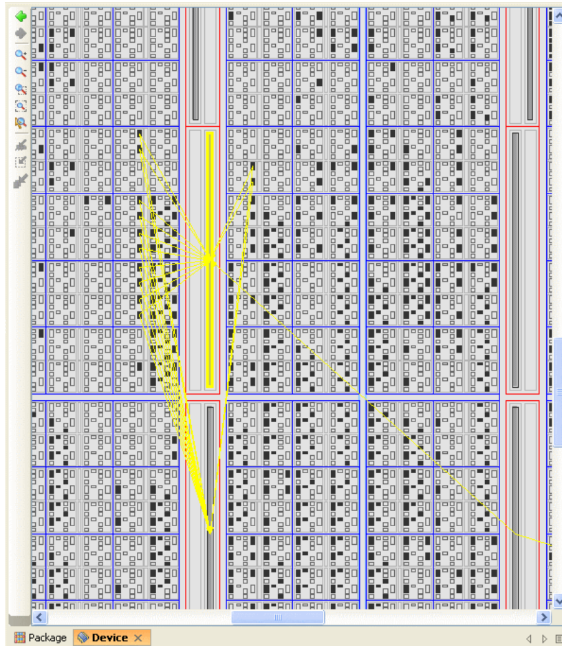
Figure 4-34: Device View with Place Instance as Rectangles
