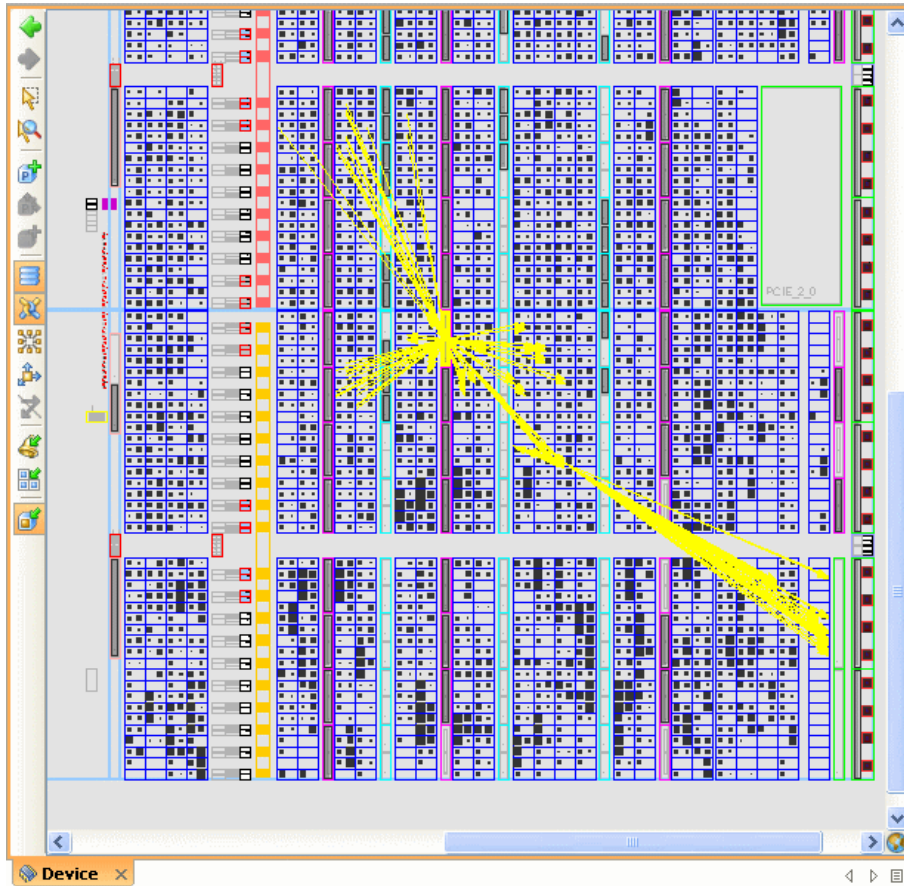
Figure 10-11: Net Connectivity in the Device View
