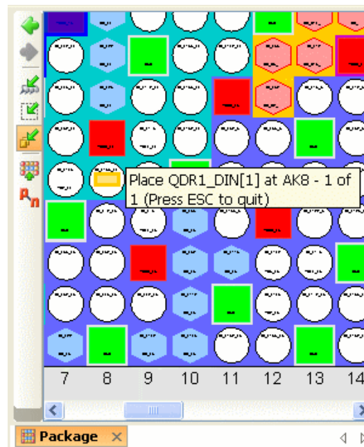
Figure 8-25: Placing I/O Ports Sequentially
