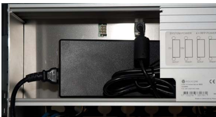
Figure 1-8 Storing room for two AC power adapters
