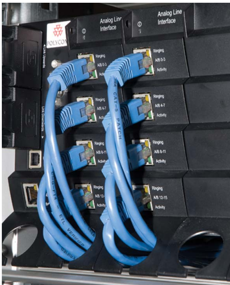
Figure 1-11 Harnessing cables to the back and out
