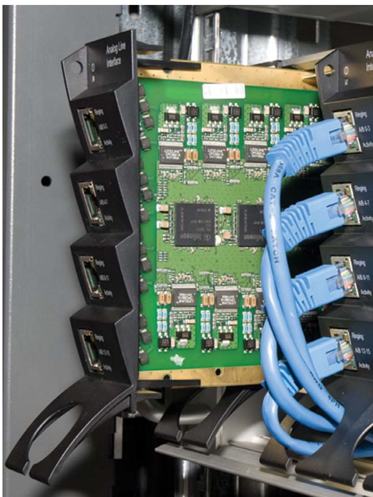
Figure 1-9 Installing Interface Cards
