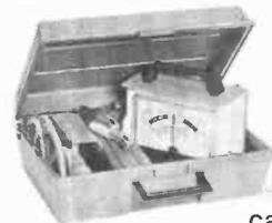
relative combustion efficiency, air-fuel ratio and percentage carbon monoxide.
