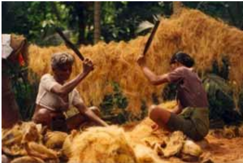
Figure 21: Manual extraction of coco fibre by beating with wooden malletsk
