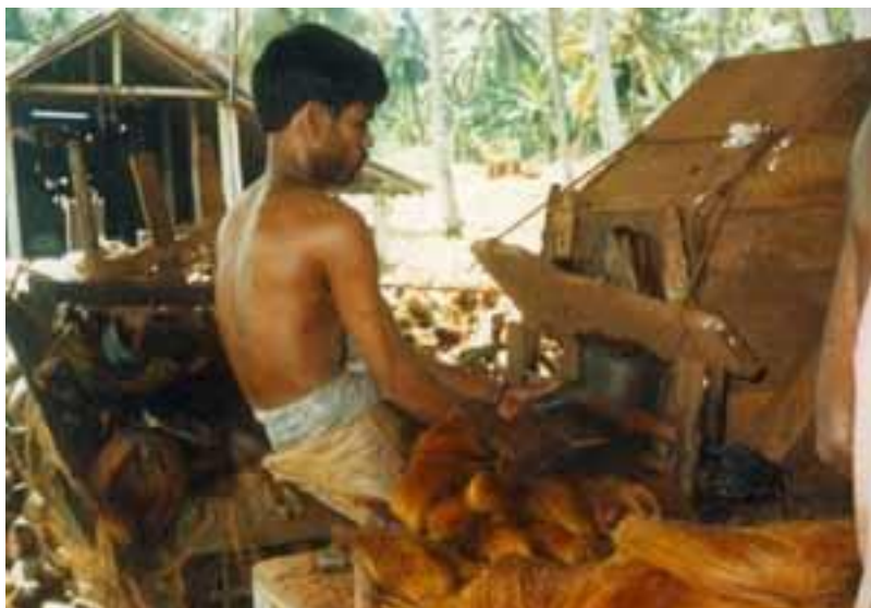
Figure 20a: Mechanical extraction of the coconut husk
