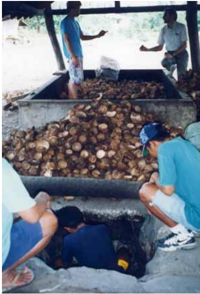
Figure 9: Semi-Direct Smoke Copra Dryer
