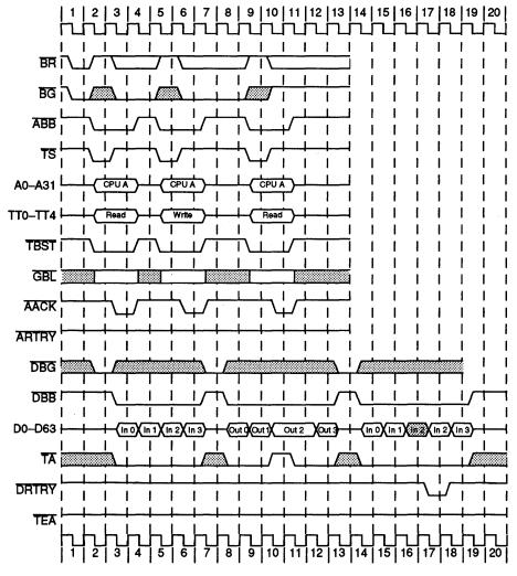
Figure 8-20. Burst Transfers with Data Delay Controls
