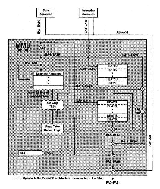
Figure 5-1. MMU Conceptual Block Diagram-32-Bit Implementations
