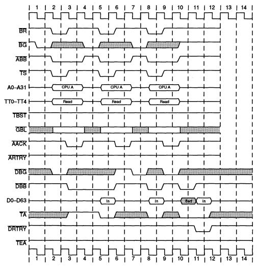
Figure 8-18. Single-Beat Reads Showing Data-Delay Controls
