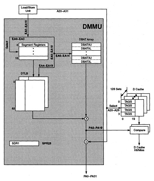
Figure 5-3. PowerPC 604 Microprocessor DMMU Block Diagram
