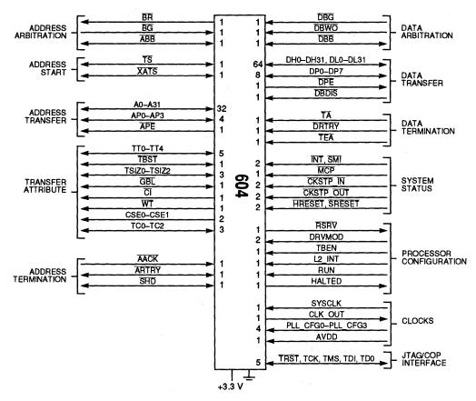
Figure 1-5. PowerPC 604 Microprocessor Signal Groups
