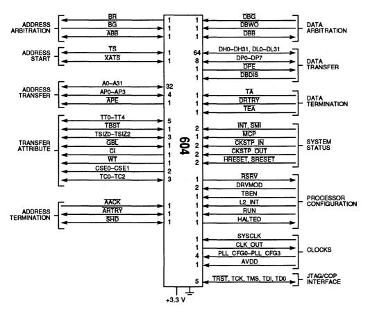
Figure 7-1. PowerPC 604 Microprocessor Signal Groups
