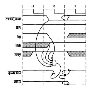
Figure 8-5. Address Bus Arbitration Showing Bus Parking
