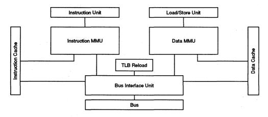
Figure 3-3. Bus Interface Unit and MMU
