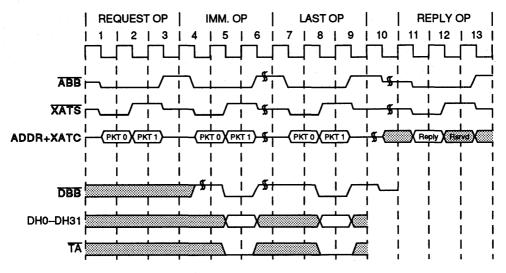
Figure 8-26. Direct-Store Interface Load Access Example
