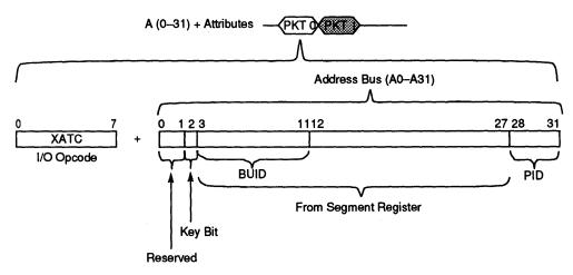
Figure 8-23. Direct-Store Operation—Packet 0
