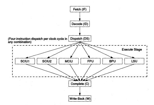
Figure 6-3. Pipeline Diagram
