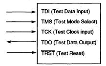
Figure 7-2. IEEE 1149.1-Compliant Boundary Scan Interface
