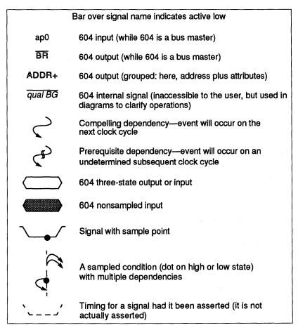
Figure 8-2. Timing Diagram Legend
