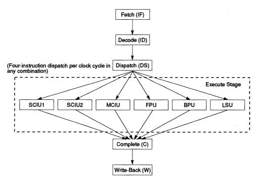
Figure 1-7. Pipeline Diagram
