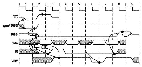
Figure 8-14. Read Burst with TA Wait States and DRTRY
