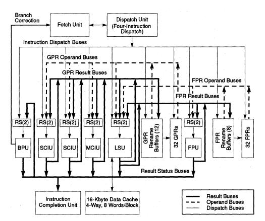
Figure 6-1. PowerPC 604 Microprocessor Block Diagram Showing Data Paths
