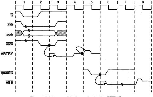
Figure 8-7. Snooped Address Cycle with ARTRY
