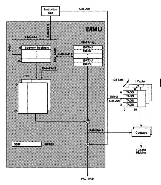
Figure 5-2. PowerPC 604 Microprocessor IMMU Block Diagram
