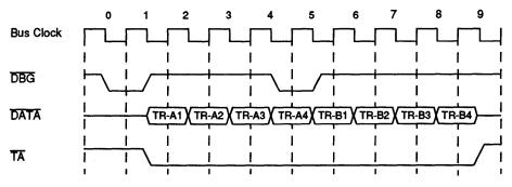
Figure 8-28. Data Transfer in Fast-L2/Data Streaming Mode
