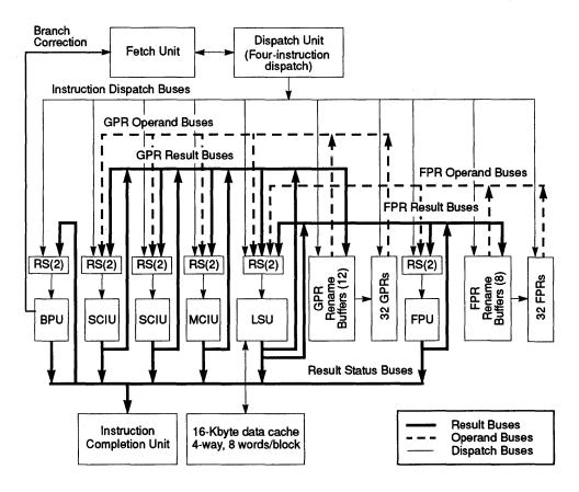
Figure 1-2. Block Diagram-Internal Data Paths
