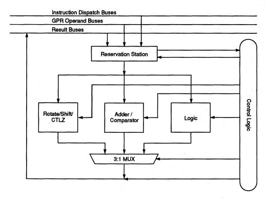
Figure 6-14. SCIU Block Diagram
