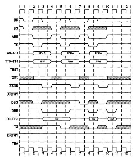
Figure 8-19. Single-Beat Writes Showing Data Delay Controls
