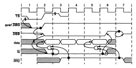
Figure 8-12. Normal Burst Transaction
