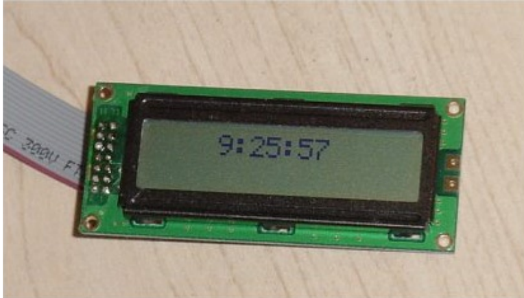
Figure 4-1. A simple character LCD clock
