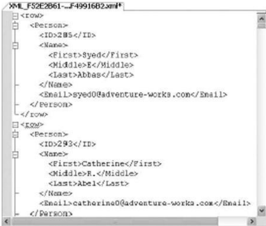
Figure 13-1. Partial Results of Retrieving Names and E-mail Addresses with FOR XML PATH
