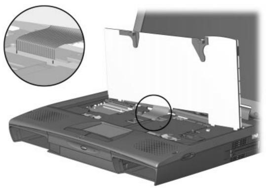
Figure 5-14. Disconnecting the keyboard Ribbon Cable
