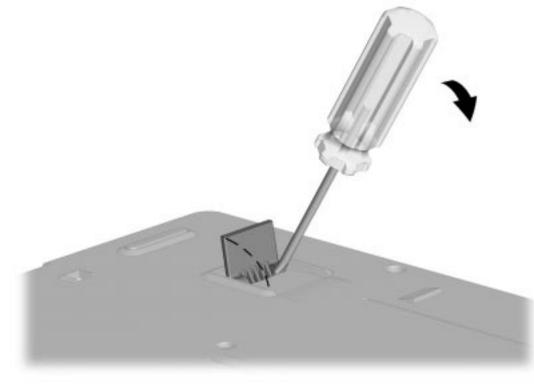
Figure 5-5. Removing the Computer Tilt Feet
