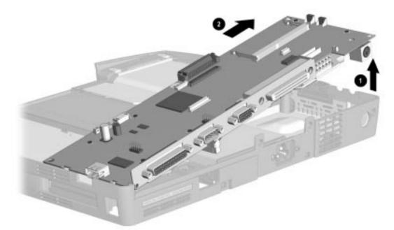
Figure 5-35. Removing the System Board
