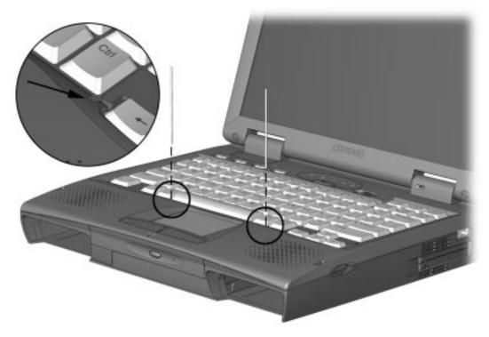
Figure 5-12. Releasing the Keyboard Latches
