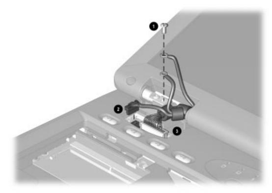
Figure 5-23. Disconnecting the Display Cables
