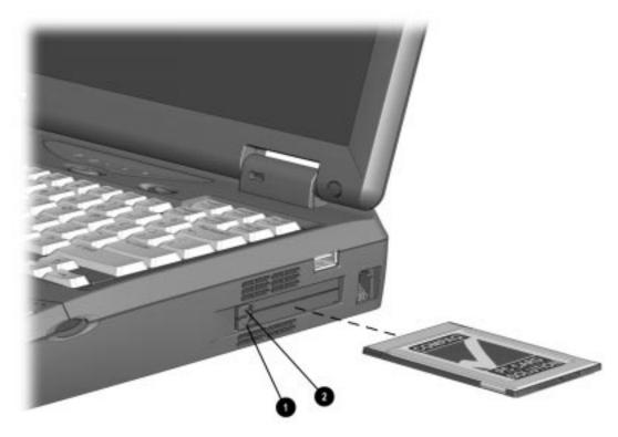
Figure 5-4. Removing the PC Card
