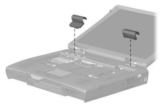
Figure 5-22. Removing the Hinge Covers
