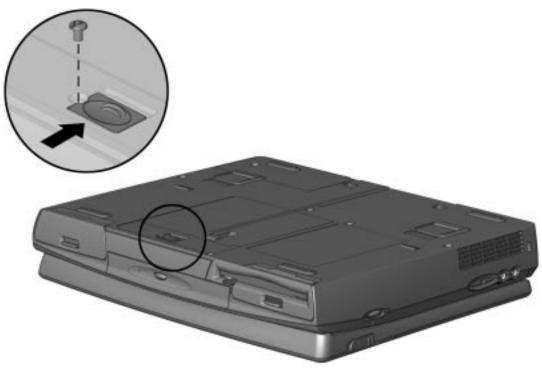
Figure 5-9. Removing the Hard Drive Cover Security Screw
