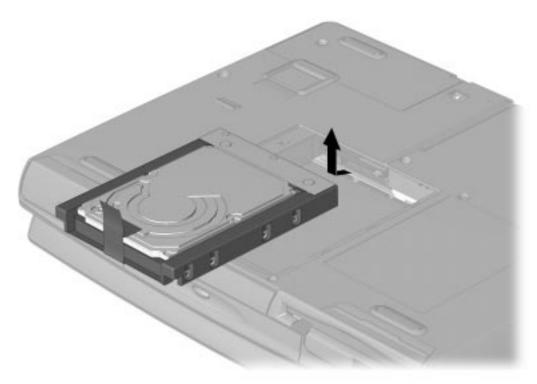
Figure 5-11. Removing the Hard Drive
