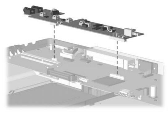
Figure 5-31. Removing the Audio Board
