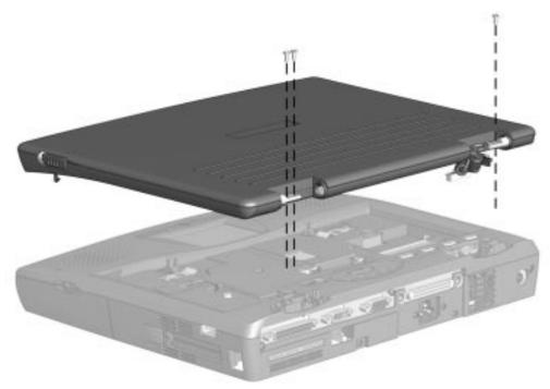
*Figure 5-24*. *Removing the Display Assembly*
