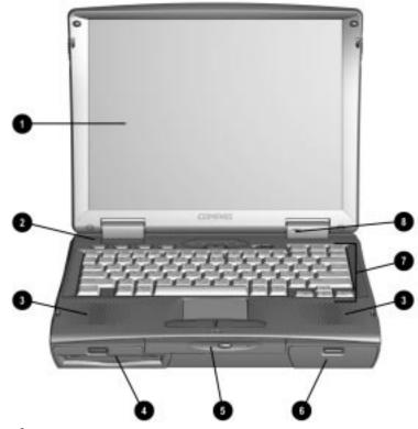
Figure 1-3. Front Components
