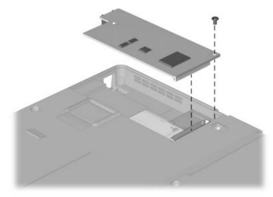
Figure 5-7. Removing the Modem Board
