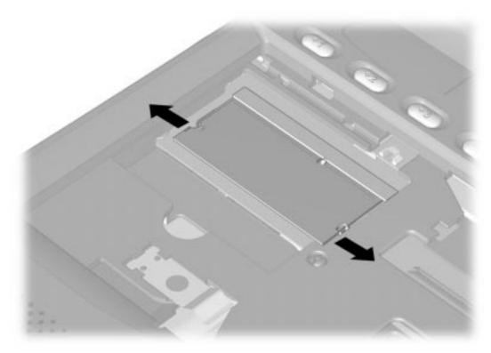
Figure 5-15. Releasing the Memory Expansion Board
