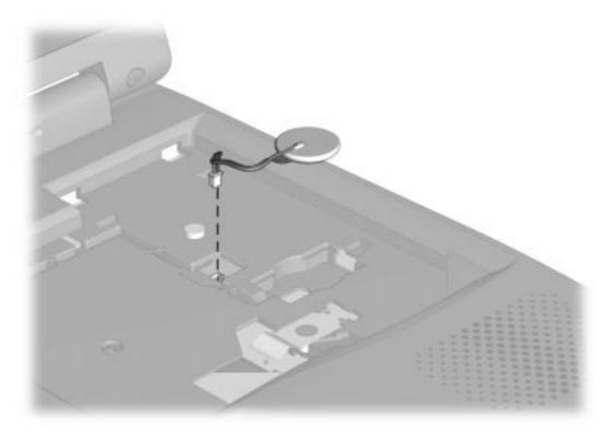
Figure 5-19. Removing the RTC Battery
