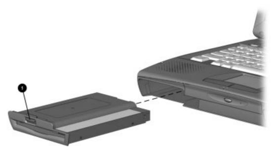
Figure 5-3. Removing the MultiBay Device
