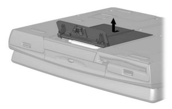
Figure 5-10. Removing the Hard Drive Cover
