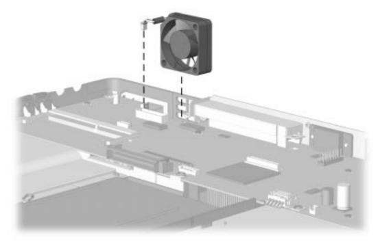
Figure 5-32. Removing the Fan
