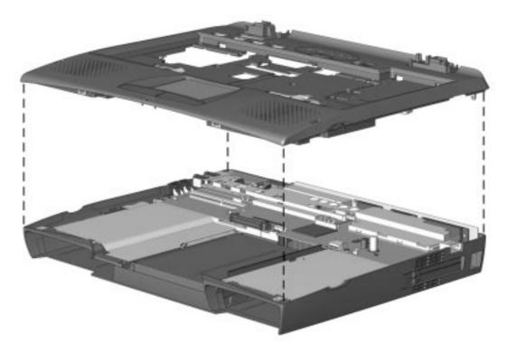
Figure 5-28. Removing the Top Cover Assembly
