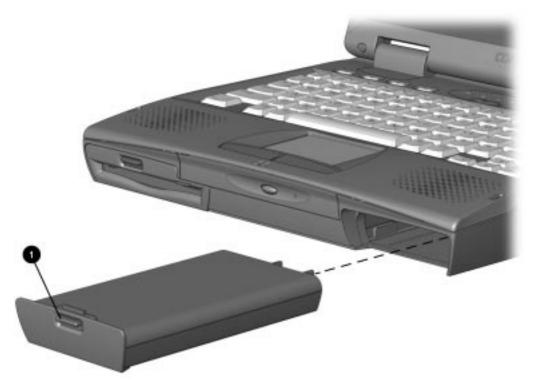
Figure 5-2. Removing the Battery Pack
