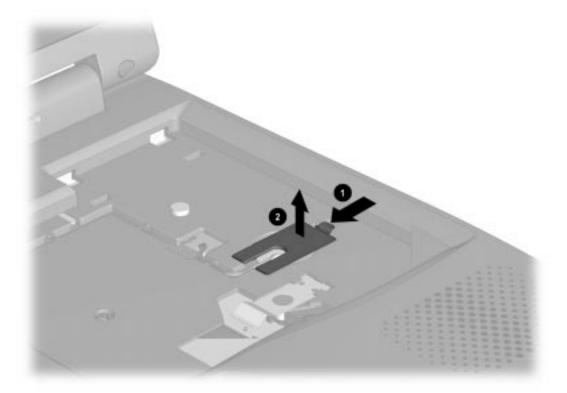
Figure 5-18. Removing the RTC Battery Cover
