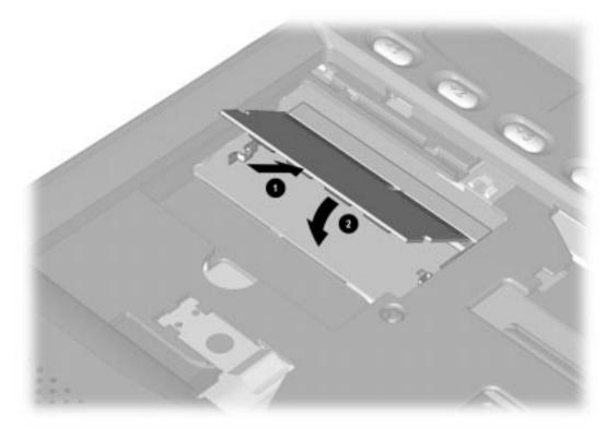
Figure 5-17. Installing the Memory Board
