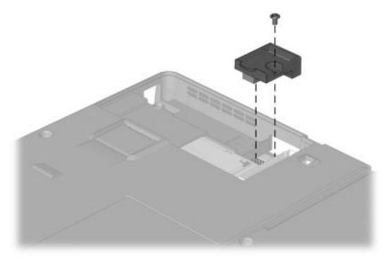
Figure 5-8. Removing the IR Module
