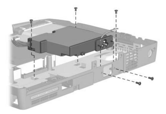
Figure 5-36. Removing the AC Adapter
