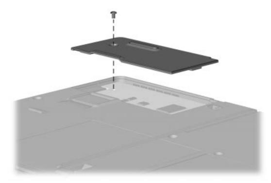
Figure 5-6. Removing the Modem Access Cover
