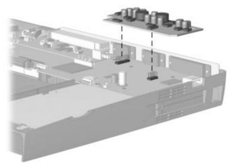
Figure 5-30. Removing the DC-DC Converter
