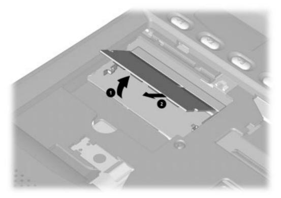
Figure 5-16. Removing the Memory Expansion Board
