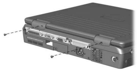
Figure 5-21. Removing the Hinge Cover Screws
