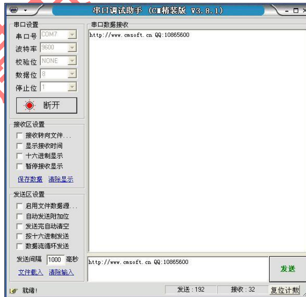
Figure 2-4. UART Loopback Test
