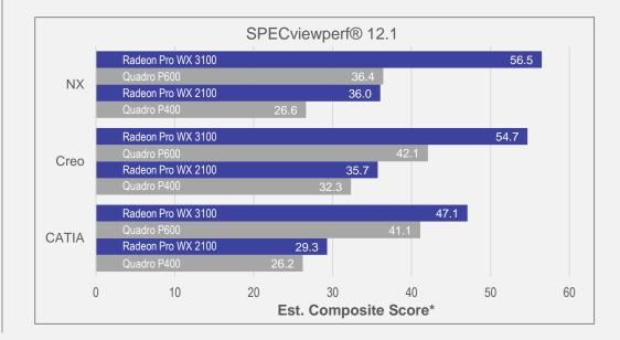
\* Testing conducted by AMD Performance Labs as of March 22nd, 2017 on a test system comprising of Intel E5-1650 v3 @ 3.50 GHz, 16GB DDR4 physical memory, Windows 7 Professional 64-bit, Radeon™ Pro WX 2100/WX 3100/NVIDIA Quadro P400/P600, AMD graphics driver 16.50/NVIDIA graphics driver 376.84. Results are an average of two runs.
