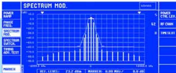
The option CMD-B43 provides measurements of spectrum due to modulation and switching according to GSM recommendations
