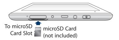
Insert the microSD card into the tablet's microSD slot until it clicks.
