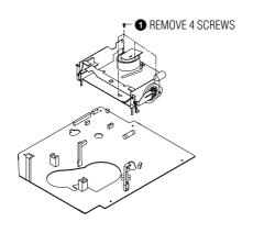
Fig. 2-6 VCR Main PCB Removal
