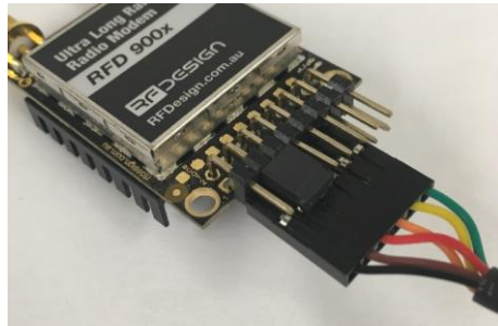
Figure 5-2: An FTDI cable connected to the RFD900x modem
