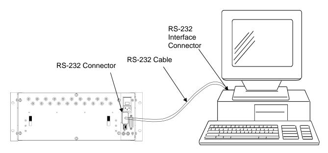
Figure 4-3, Using the RS-232 Interface
