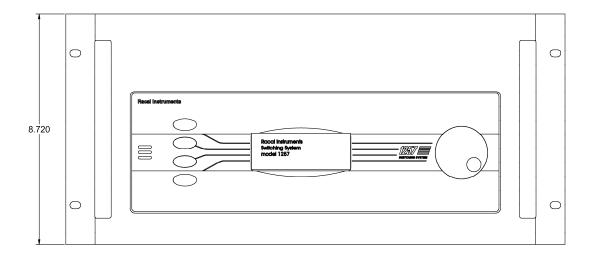
Figure 1-7, 5U Front Panel Display
