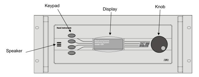
Figure 3-1, Front-Panel Controls
