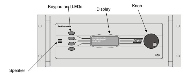
Figure 1-2, 1257 Features, Front Panel
