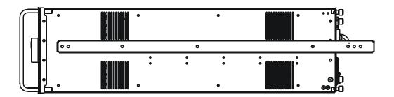
Figure B-1, Installing the Slide Kit
