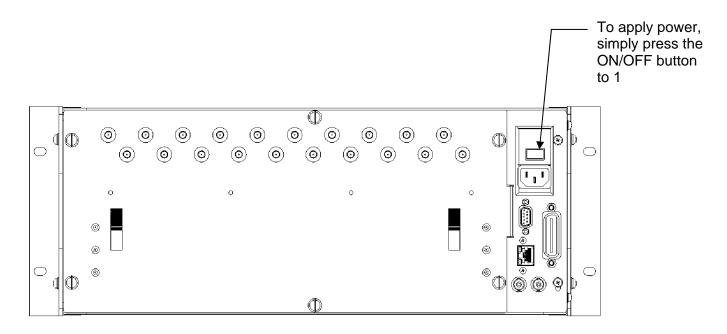
Figure 2-3, Activating Main AC Power
