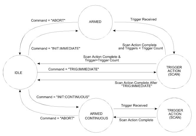
Figure 7-1, State Transition Diagram For Arming and Triggering the 1257
