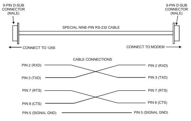
Figure 4-4b, Using the 1257 with a Modem
