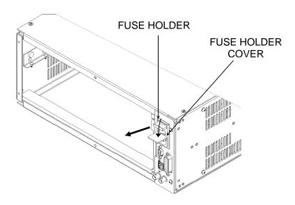
Figure 2-1, Changing Fuse for Main AC Power
