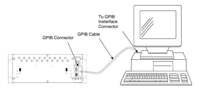
Figure 4-2, Using the GPIB Interface
