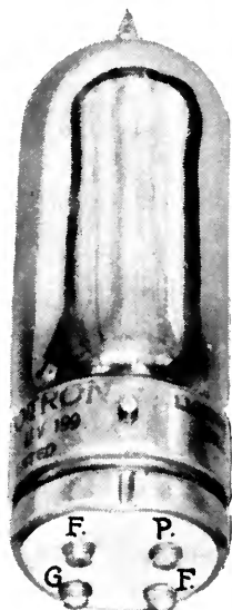
FIG. 3 Showing arrangement of contacts on the UV-199
