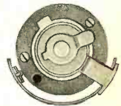
Illustrating the complete working mechanism of the control, showing traveling position of contact shoe on the resistance element.
