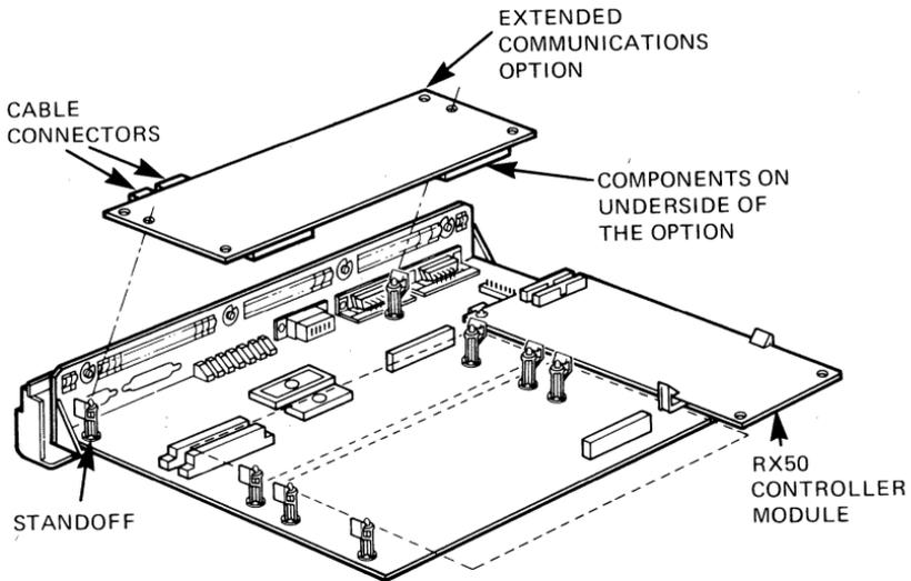
**Installing the Extended Communications Module
