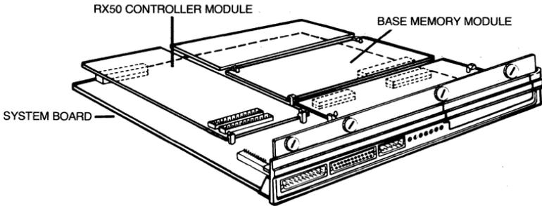
**Installing a Base Memory Module
